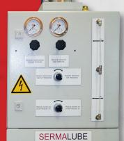
The micro-lubrication system SERMALUBE® has been designed and developed by SERMAS® for optimum lubrication for high-speed cutting applications (sheet, plate, ingot, billets) and surfacing aluminum plates.
